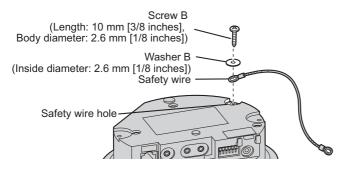
the bracket and the camera are securely mounted.
